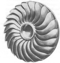
Fig. 8. Inlet and discharge sides of the runner of a Turgo impulse turbine.
